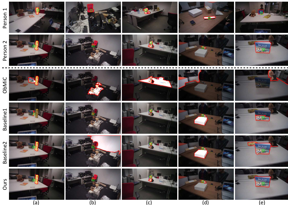
Figure 4. Segmenting Objects of Joint Attention: Examples. Red boundaries indicate jointly-attended object segments and green circles describe points of gaze. The first two rows describe the ground truth segments for the two input videos. The remaining rows show segmentation results in the second video.
